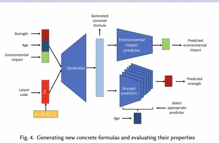
Fig. 4. Generating new concrete formulas and evaluating their properties
